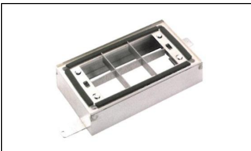
Telescopic frame for air passage box for ground installation, max. air volume: 30 m³/h consists of 1 mounting frame, 1 sliding frame, 1 load distribution element, 1 flush-frame with grille retaining clips and cover plate, 4 distance screws
